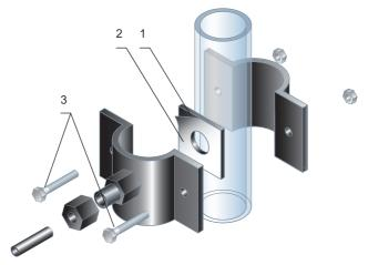
Figure 9a. Drain saddle components
