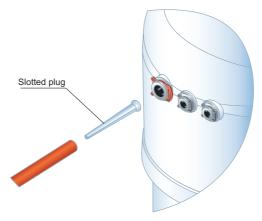
Figure 10. Slotted plug installation
