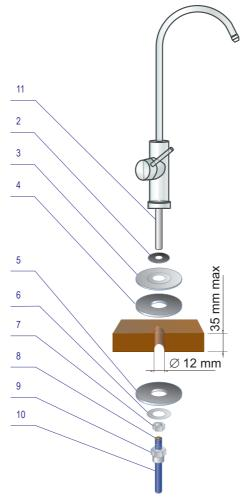
Figure 8. Tube connecting to the clean water faucet procedure
