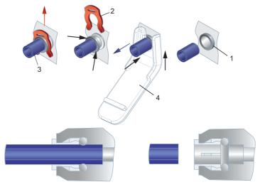
Figure 7. Disconnection of JG tubes
