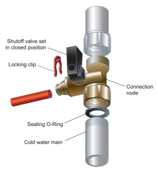
Figure 5. Connection node installation scheme
