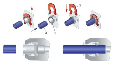
Figure 6. Connection of JG tubes
